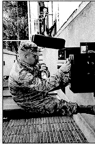
Airman 1st Class BeauX Hebert, 14th Medical Operations Squadron Bioenvironmental Technician, assembles an MMX machine June 20, 2017, at Columbus Air Force Base, Mississippi. The MMX is a vacuum that takes in air and runs it through water which can then be tested for chemicals and biological material.
